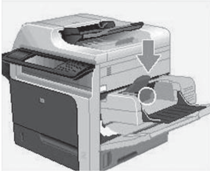
Figure 3-18 Test the PS1802 envelope feeder paper sensor
