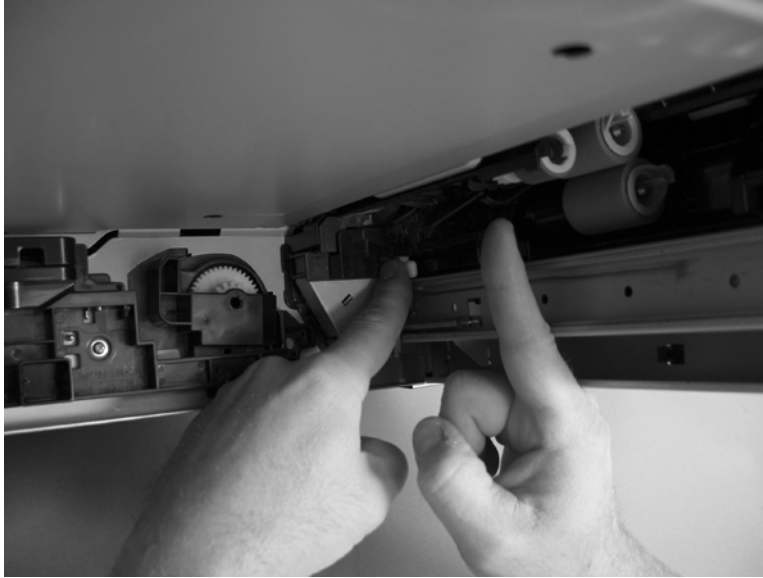
Figure 3-21 Test the PS107/PS907 Tray 2 paper surface sensor
