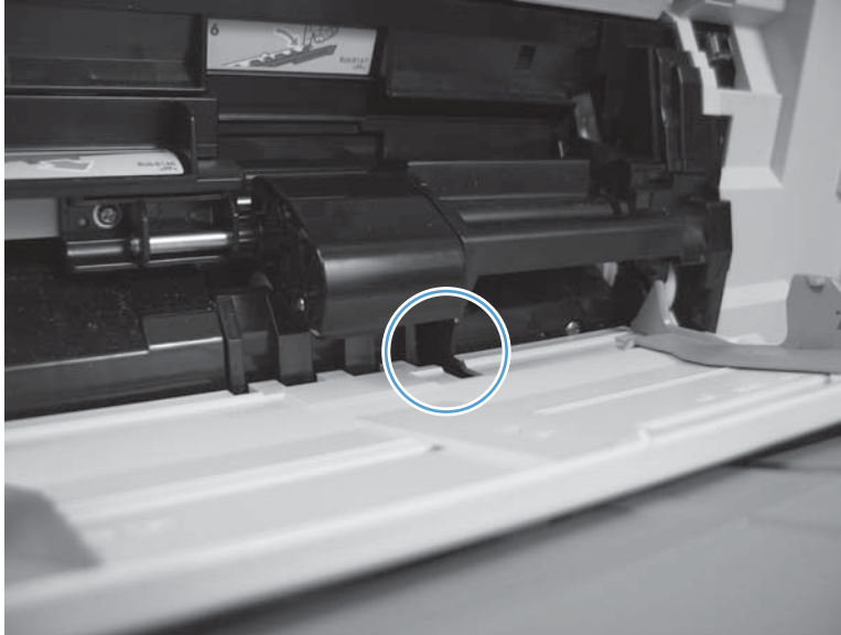
Figure 3-19 Test the PS114 Tray 1 paper sensor
