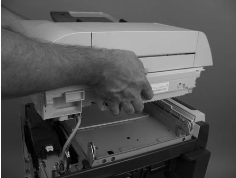
Figure 2-86 Remove the document feeder (4 of 4)
