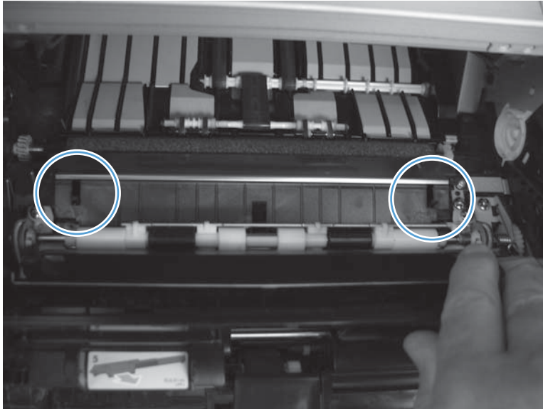
Figure 3-11 Test the PS106/108 paper width sensors
