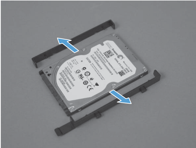
Figure 2-40 Remove the encrypted HDD (5 of 5)
