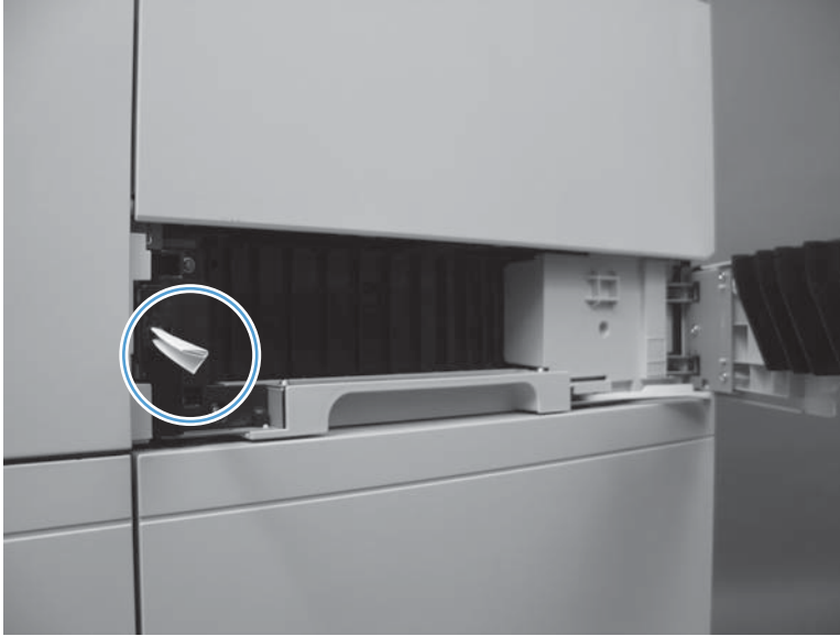
Figure 3-4 Test the SW105 right upper door switch
