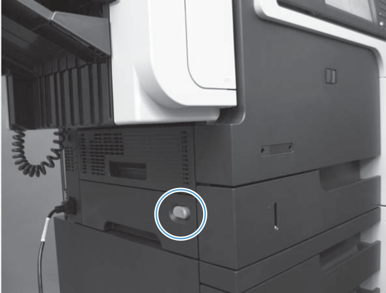
Figure 3-27 Test the SW1 power switch
