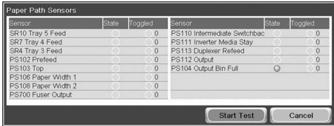
Figure 3-31 Paper path sensors test screen
