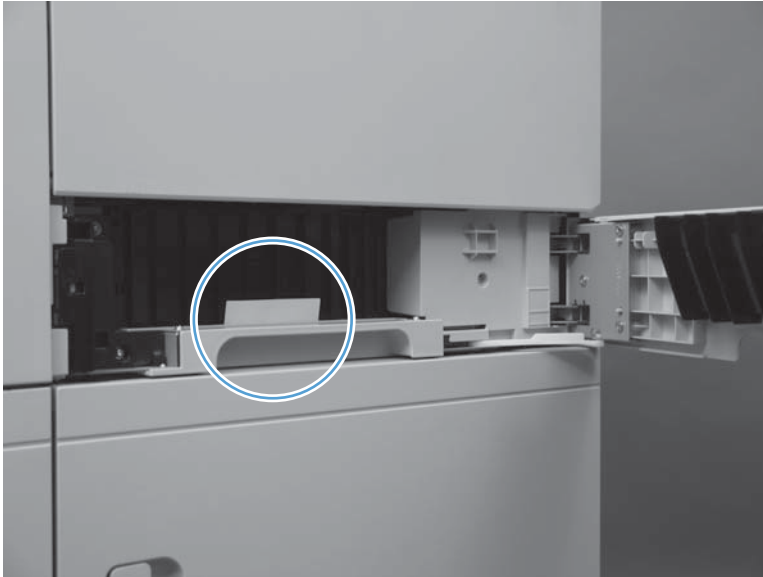
Figure 3-8 Test the SR4 Tray 3 feed sensor
