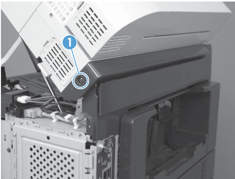
Figure 2-79 Remove the document feeder hinge cover (1 of 3)
