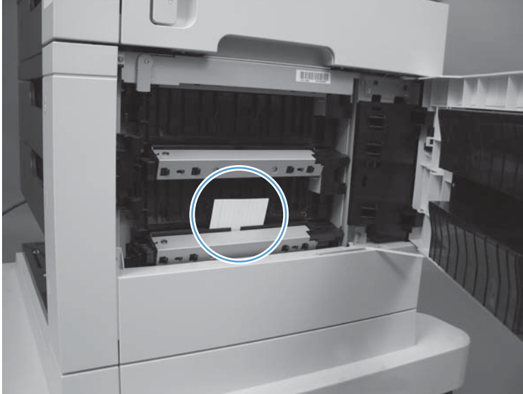
Figure 3-6 Test the SR10 Tray 5 feed sensor
