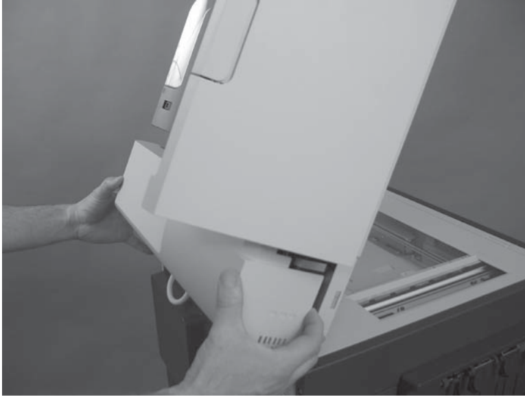
Figure 2-182 Remove the document feeder rear cover (5 of 5)
