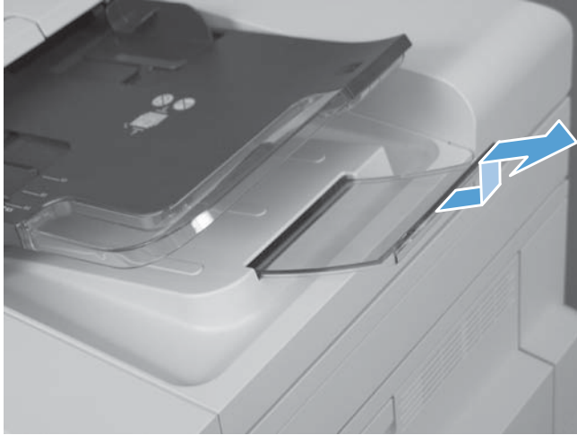
Figure 2-42 Remove the document feeder tray extender
