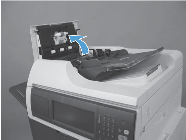
Figure 2-174 Remove document feeder front cover (1 of 4)
