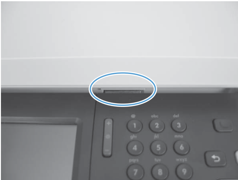
Figure 2-19 Correct installation of the control panel
