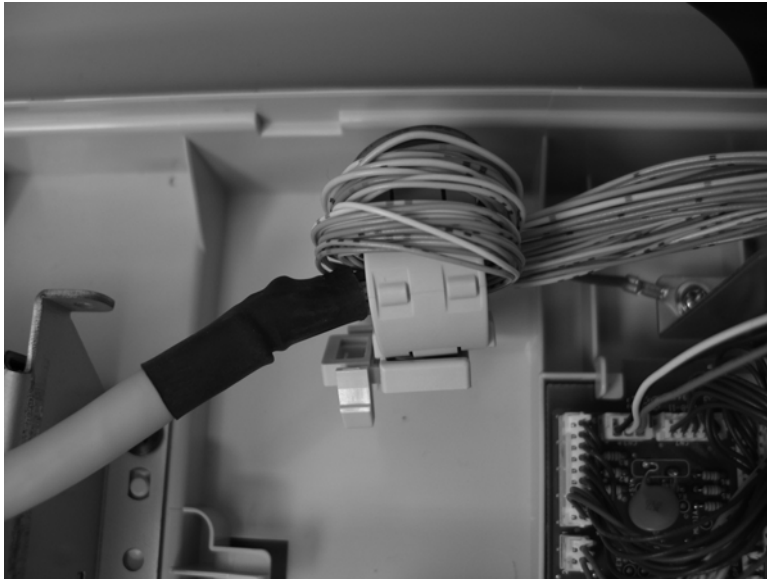
Figure 2-192 Reinstall the document feeder cable
