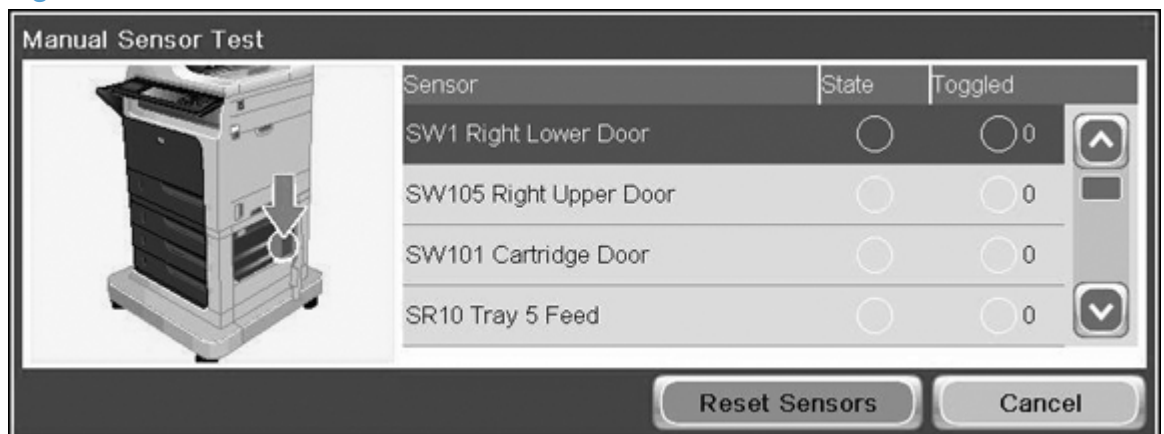
Figure 3-2 Manual Sensor Test screen
