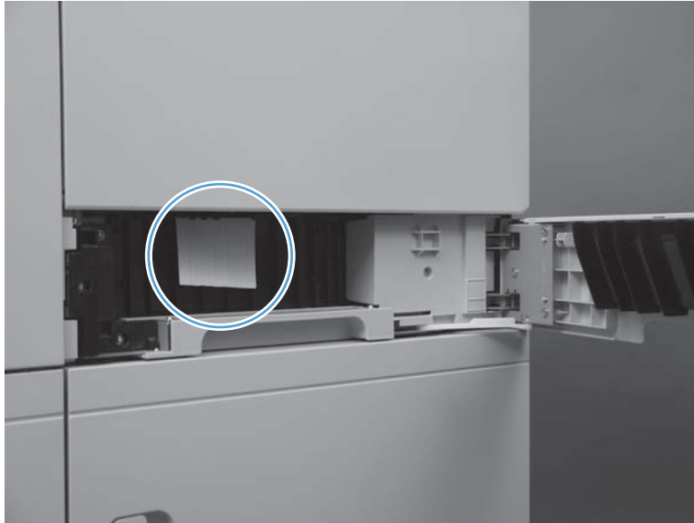
Figure 3-9 Test the PS102 pre-feed sensor
