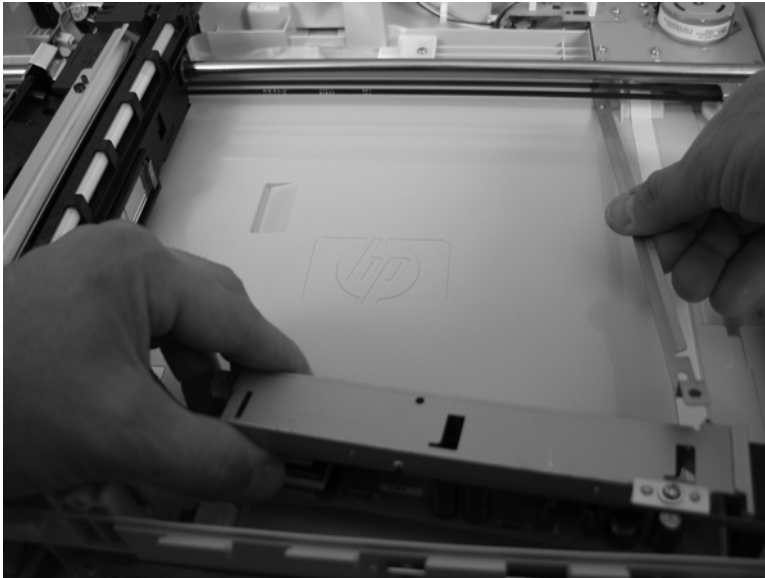
Figure 2-219 Remove the inverter (2 of 2)
