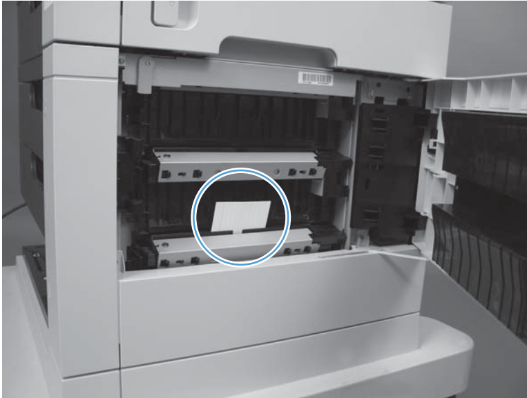
Figure 3-25 Test the SR10 Tray 5 feed sensor
