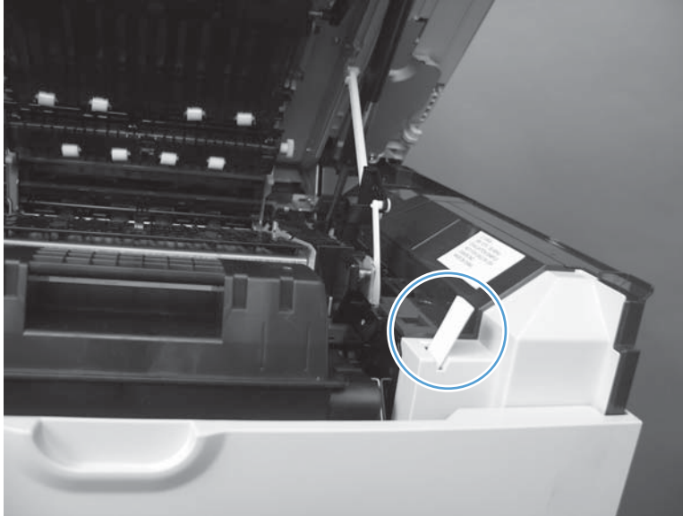
Figure 3-5 Test the SW101 cartridge door (top cover) switch
