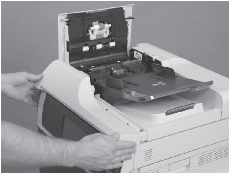
Figure 2-177 Remove document feeder front cover (4 of 4)
