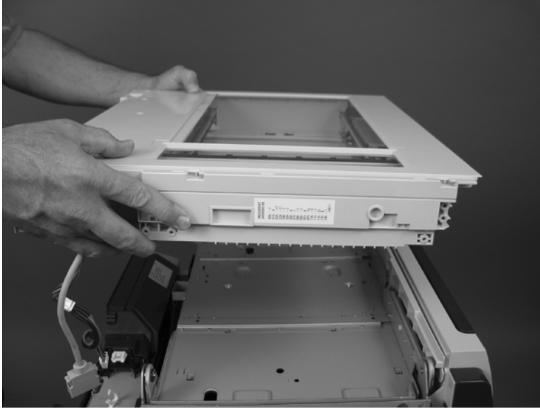
Figure 2-204 Remove the scanner assembly (4 of 4)
