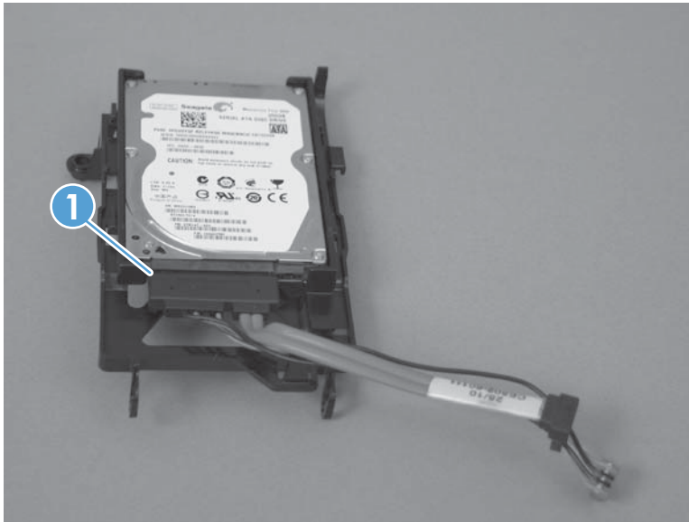
Figure 2-38 Remove the encrypted HDD (3 of 5)
