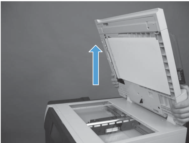
Figure 2-171 Remove the document feeder scanner lid (3 of 3)
